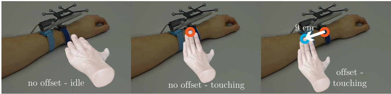
Figure 5: Participant's view during the haptic discrimination task (cloth cover removed for better visibility). Left: Idle Handifact before touching. Middle: Medium Handifact touching. Right: Medium Handifact touching in the Offset condition.
