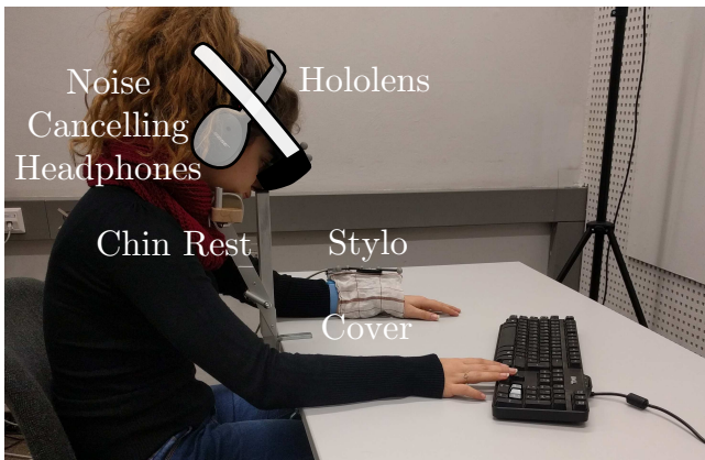
Figure 4: Setup during the haptic discrimination task.
